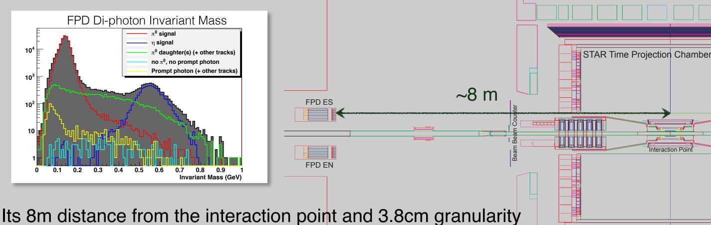
Its 8m distance from the interaction point and 3.8cm granularity results in high detection efficiency for π<sup>0</sup> with energies of up to 55 GeV.
