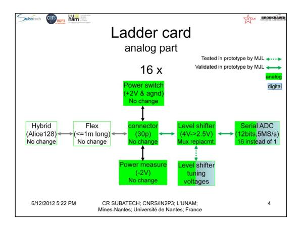
The only change (compared to old SSD) in the analog part is the ADC.
