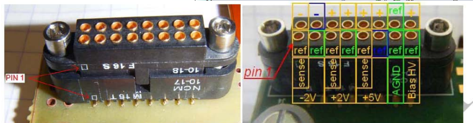
Figure 17: Nicomatic power connector cabling
