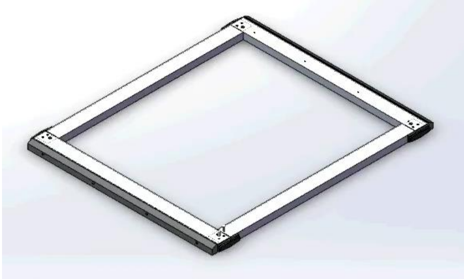
Figure 47: A sketch of the temporary wire transfer frame. The inner size for the box is 76.2 x 90.0 cm and the size of the material is 3.0 x 6.0 x 0.3 cm.
