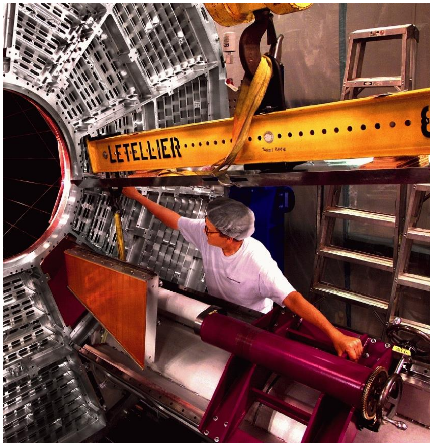
Figure 65: The original sector insertion tool. The sector must fit through the hole in the end-wheel, rotate, and finally pull back into place over a pair of alignment pins (tooling balls) that are located inside the TPC.
