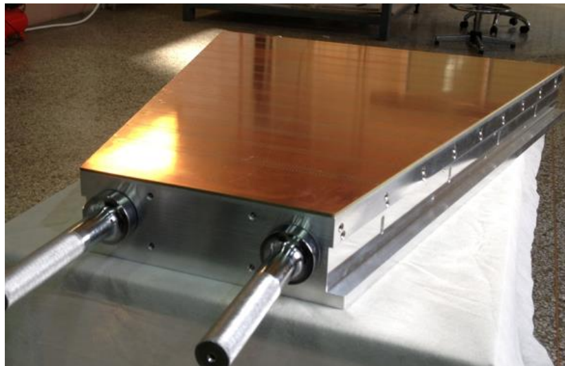
Figure 50: The strongback with the pad plane glued.
