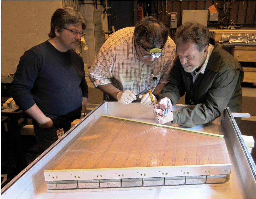
Figure 58: Experts examining a spare inner sector for the TPC. Note the old style padplane with electronics cards (ABDB boards) mounted along the edge of the sector. Normally the spare sectors (STAR has two spare sectors) are sealed in a storage box and kept under dry nitrogen.
