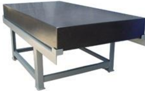
Figure 62: A typical Grade A inspection plate; otherwise known as a granite table. Typical dimensions are 6 feet by 4 feet by 8 inches, although the tables are available in many different sizes.
