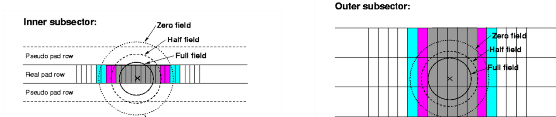
Figure 34: Simulations of the effective pad response function for pads on the inner and outer TPC padplanes. The inner pads were assumed to be 3.35 mm wide and the outer pads 6.7 mm wide. The circles show the 3-sigma limit for the pad response function convoluted with the diffusion limit for particles that drift the full distance from the CM to the padplane. P10 gas is assumed. The different circles show the different response that is recorded when the B field is set to 0.0, 0.25 T, or 0.5 T. [4]
