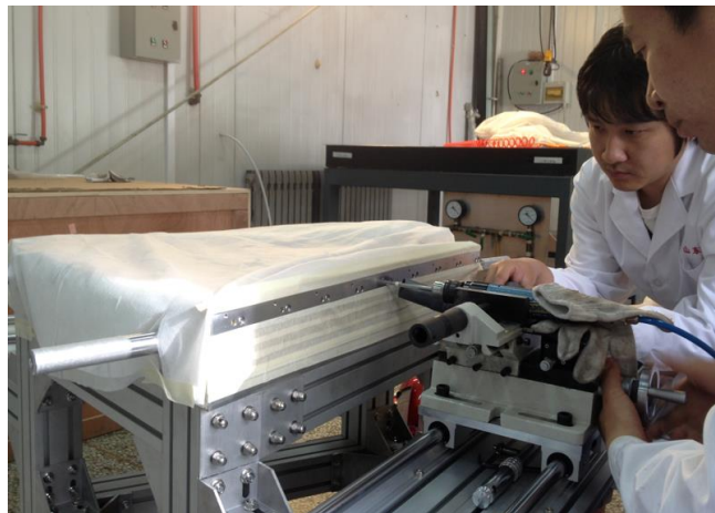
Figure 56: Drilling & pinning on side wire mounts
