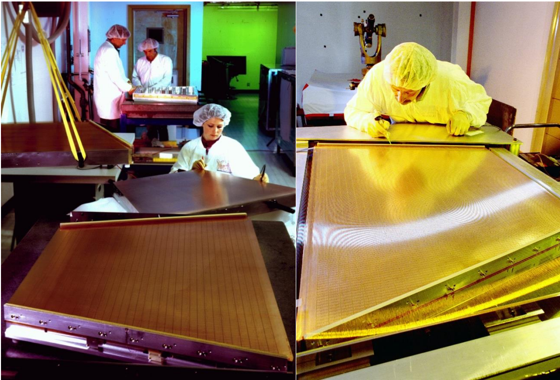
Figure 41: Outer sector MWPCs under construction in Berkeley (circa 1995).
