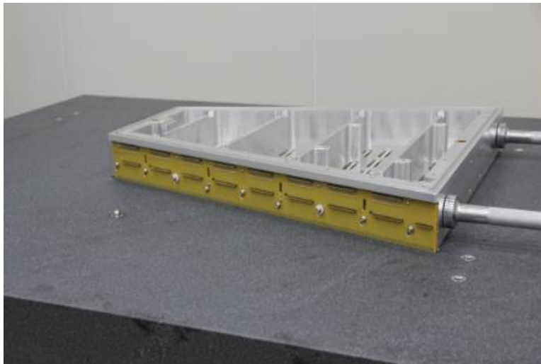
Figure 52: The anode wire mounts were glued to the strongback with epoxy.
