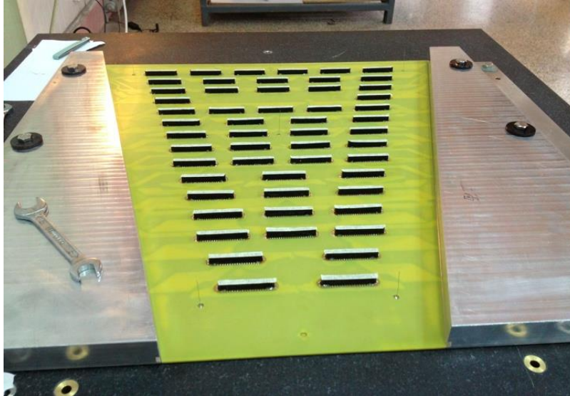
Figure 49: Padplane on granite table held flat by the suction of a vacuum system.
