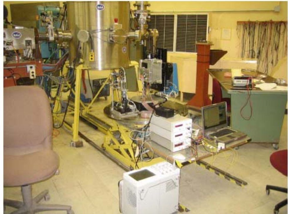
Figure 1 SEUTF at BNL. The MimoStar2 test setup is visible in the front. Visible in the back is vacuum chamber open to allow fixing the device under test.
