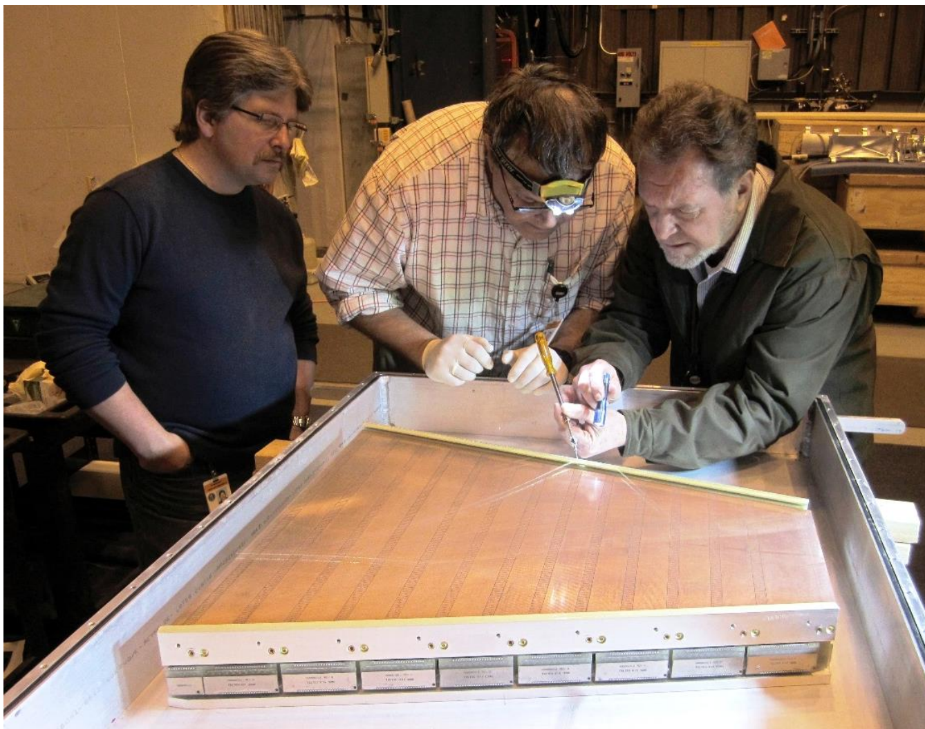
Figure 40: Experts examining a spare inner sector for the TPC. Note the old style pad plane with electronics cards (ABDB boards) mounted along the edge of the sector. Normally the spare sectors (STAR has two spare sectors) are sealed in a storage box and kept under dry nitrogen.
