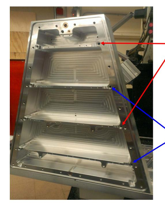
TwinAX connectors to pulse the Gating Grid (2 places, total). Vacuum feedthroughs with O-ring seal.
