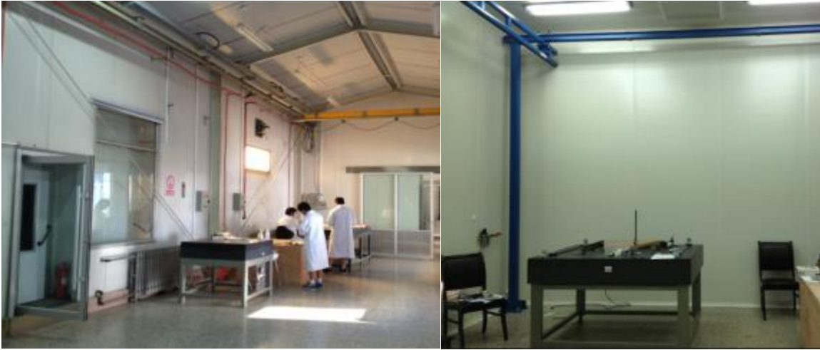
Figure 64: Experimental hall with two granite tables (left) and clean room with crane and granite table (right) for MWPC production at SDU.
