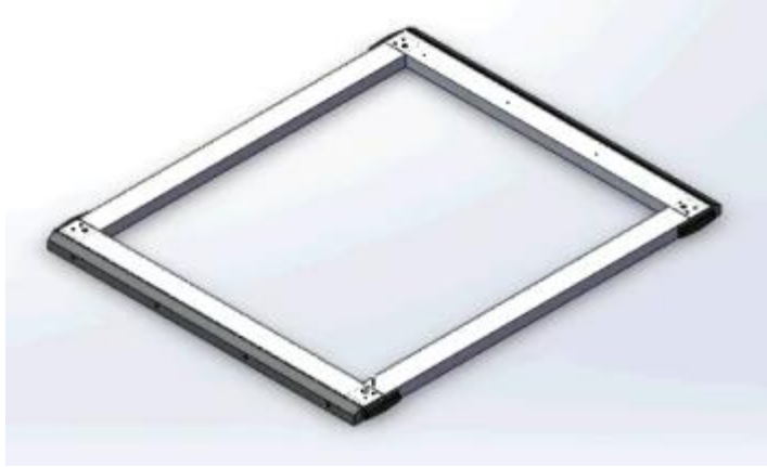
Figure 74: A sketch of the temporary wire transfer frame. The inner size for the box is 76.2 x 90.0 cm and the size of the material is 3.0 x 6.0 x 0.3 cm.
