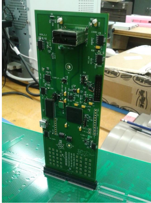
Figure 91: Pre-prototype iFEE (ppFEE) electronic card shown plugged into the padplane
