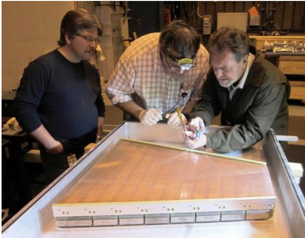
Figure 55: Experts examining a spare inner sector for the TPC. Note the old style padplane with electronics cards (ABDB boards) mounted along the edge of the sector. Normally the spare sectors (STAR has two spare sectors) are sealed in a storage box and kept under dry nitrogen.
