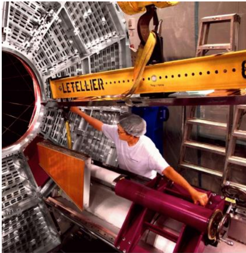
Figure 93: The original sector-mounting tool. The sector must fit through the opening in the end-wheel, rotate, and finally pull back into place over a pair of alignment pins (tooling balls) that are located inside the TPC.
