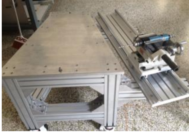
Figure 83: The drill/pinning fixture designed at SDU
