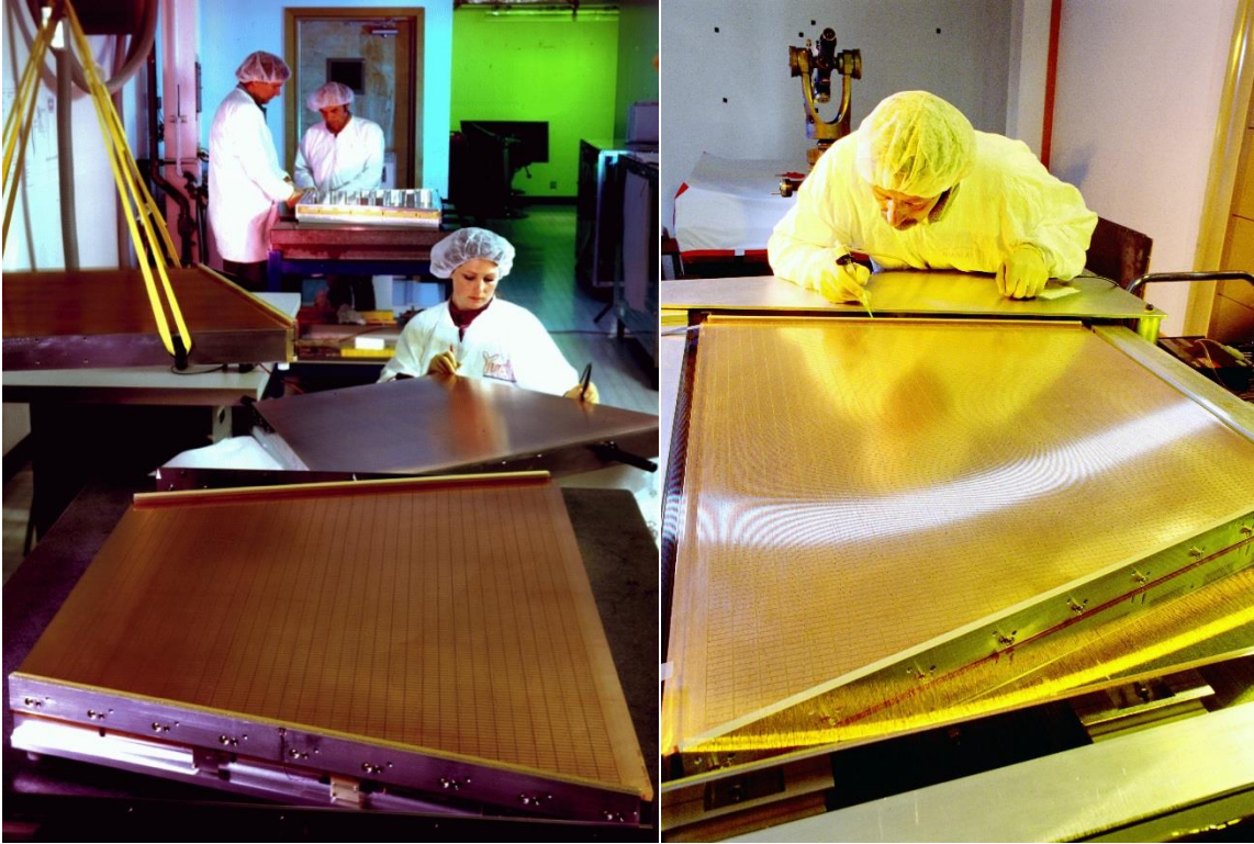
Figure 63: Outer sector MWPCs under construction in Berkeley (circa 1995).
