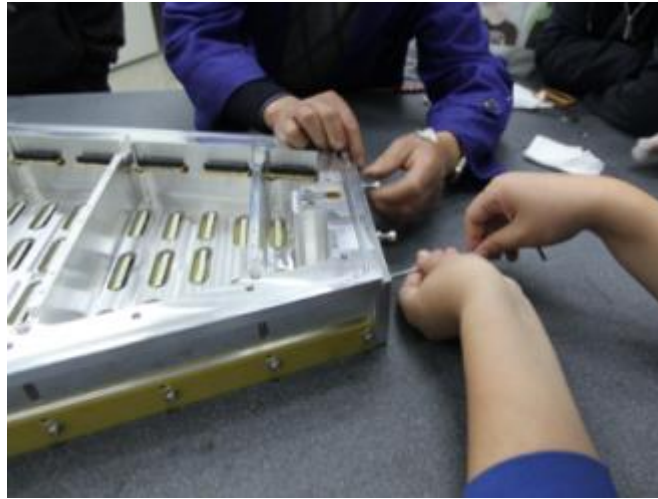
Figure 81: Attaching shield & gated wire mounts to strongback
