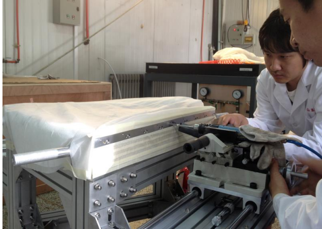
Figure 76: Drilling & pinning on side wire mounts
