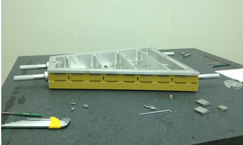
Figure 73: Attaching shield & gated wire mounts to strongback
