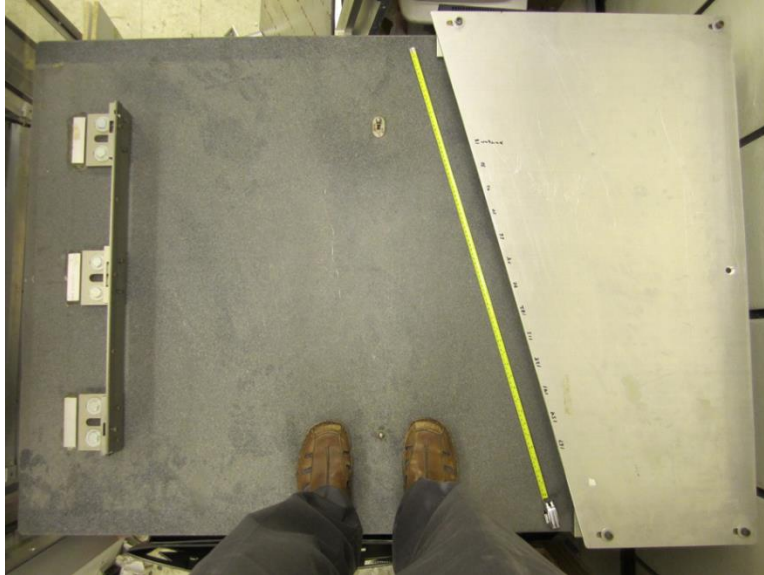
Figure 59: Top view of a granite table with one of the wire alignment combs exposed. The second comb lies under the aluminum shield on the right. Scale: the yellow portion of the tape is 1 meter long.
