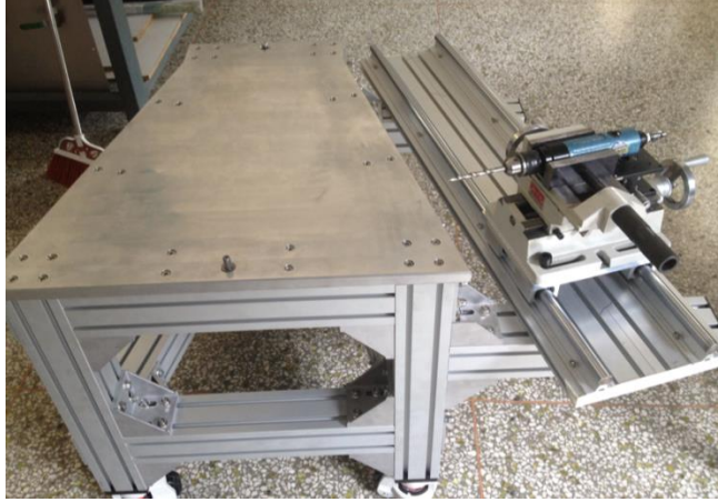
Figure 75: The drill/pinning fixture designed at SDU
