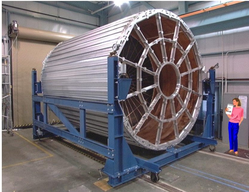
Figure 33: The STAR TPC during construction at LBL. The tracking volume of the TPC is 4 meters in diameter and 4.2 meters long. The photo shows how each end of the TPC is divided into 12 super-sectors and each super-sector is divided into an inner and an outer readout sector.
