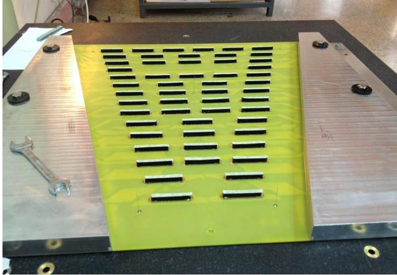
Figure 69: Padplane on granite table held flat by the suction of a vacuum system.
