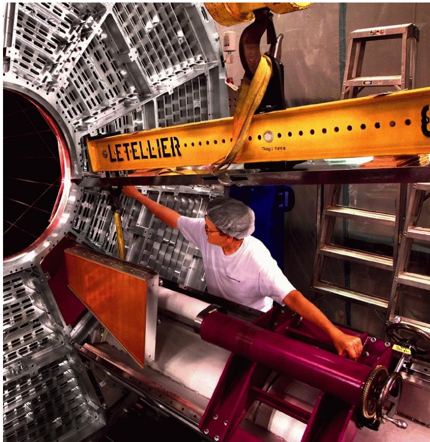
Figure 77: The original sector insertion tool. The sector must fit through the hole in the end-wheel, rotate, and finally pull back into place over a pair of alignment pins (tooling balls) that are located inside the TPC.
