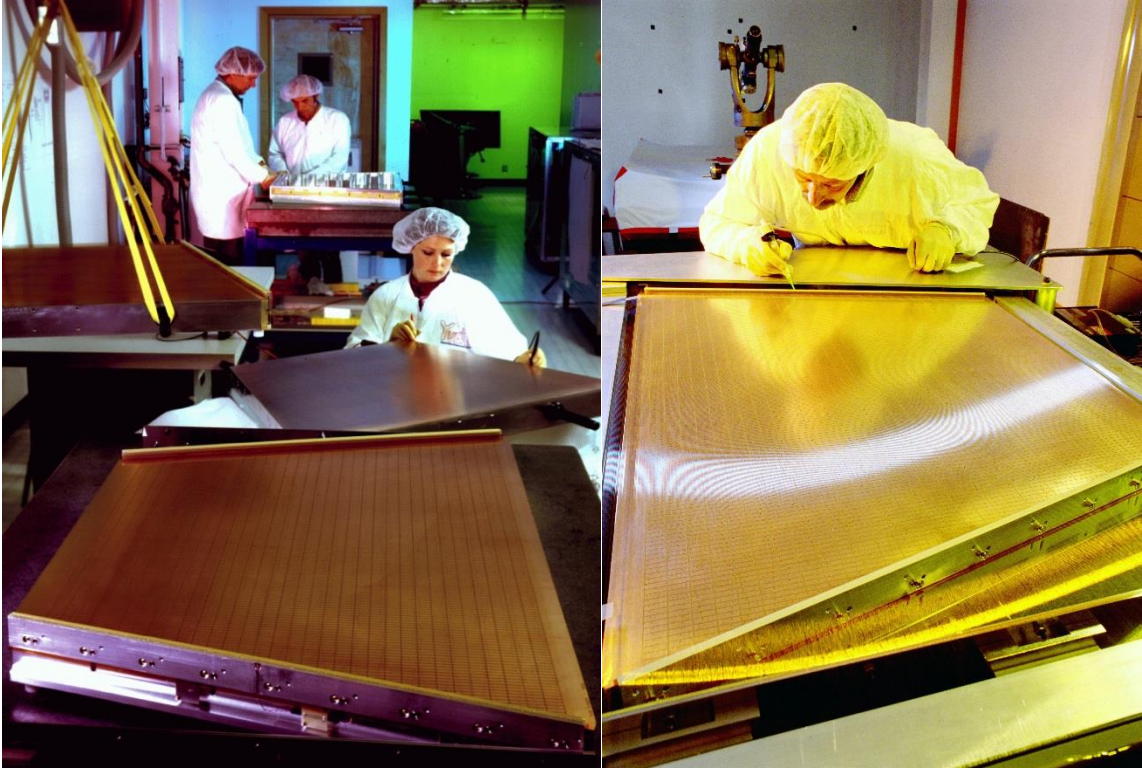
Figure 61: Outer sector MWPCs under construction in Berkeley (circa 1995).
