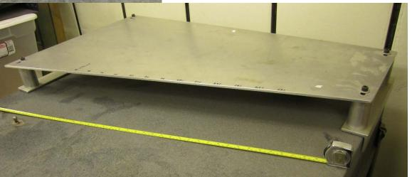
Outside edge of spacers are aligned with the edge of the granite table
