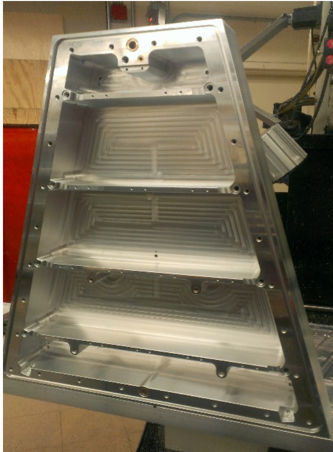
Figure 54: A prototype inner sector strongback is shown during fabrication at the University of Texas (circa 2013). The sector was machined out of a single piece of aluminum. Dimensions are: ~27 inches tall, ~25 inches wide and weight 73 lbs. The sector is viewed from the backside; the side upon which the electronics and cooling manifolds will eventually be mounted.
