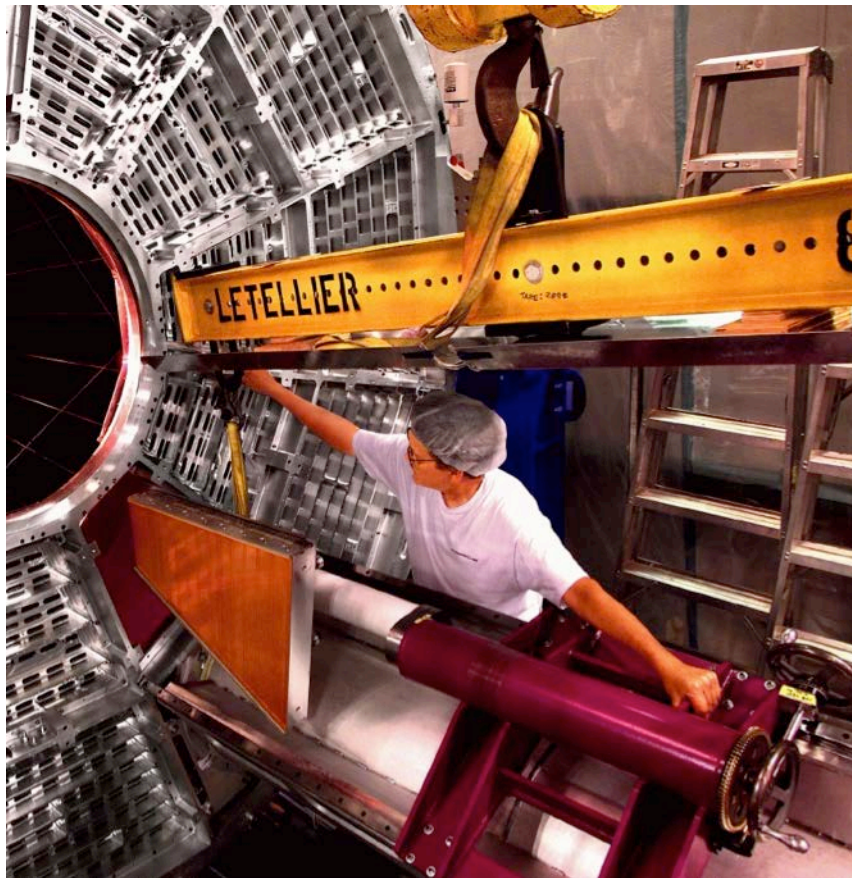
Figure 91: The original sector-mounting tool. The sector must fit through the opening in the end-wheel, rotate, and finally pull back into place over a pair of alignment pins (tooling balls) that are located inside the TPC.
