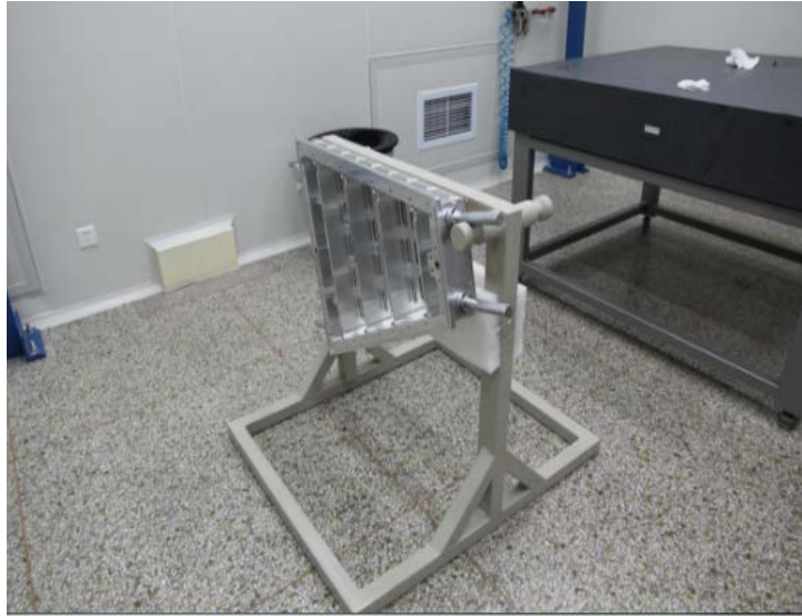
Figure 75: Gluing stand for anode wire mount and granite table.
