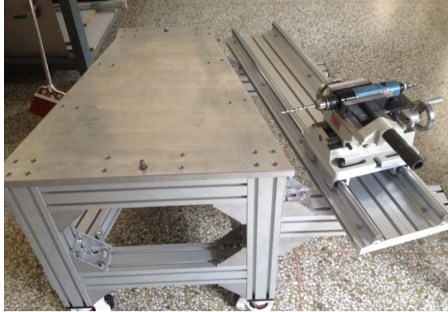
Figure 79: The drill/pinning fixture designed at SDU
