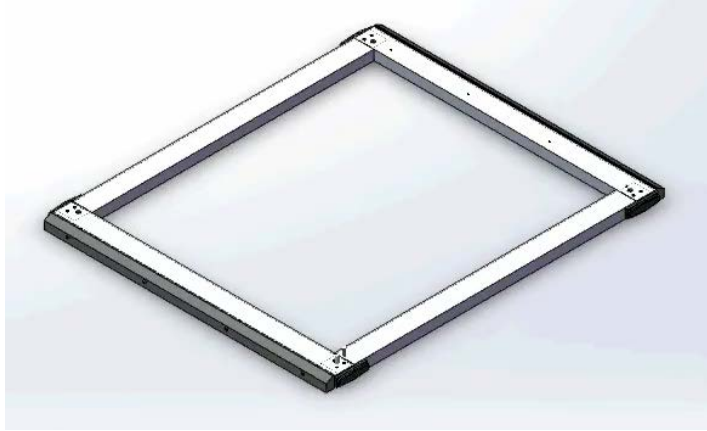
Figure 70: A sketch of the temporary wire transfer frame. The inner size for the box is 76.2 x 90.0 cm and the size of the material is 3.0 x 6.0 x 0.3 cm.
