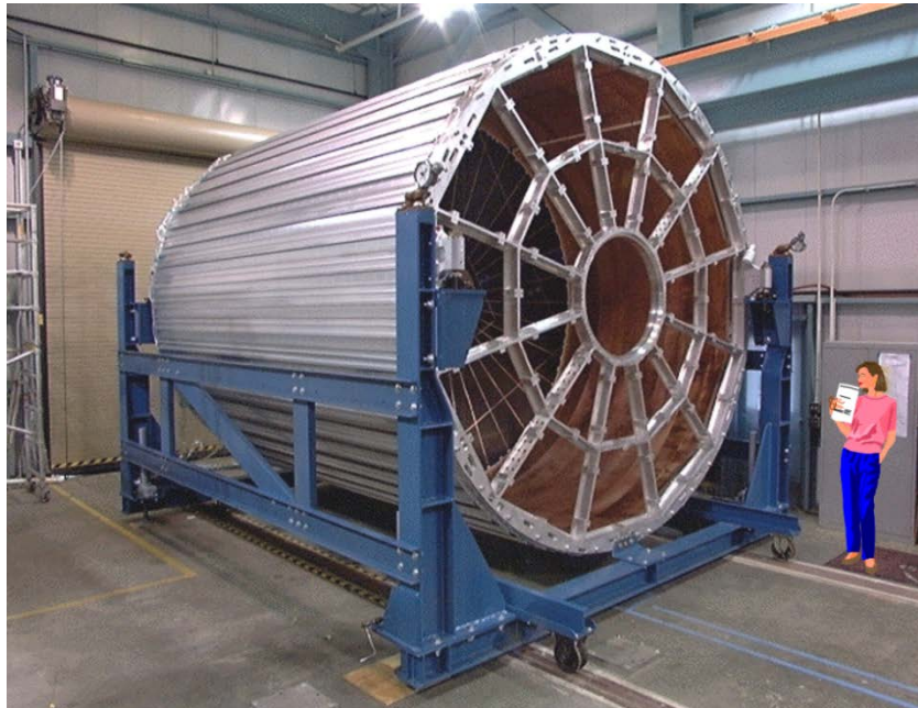
Figure 36: The STAR TPC during construction at LBL. The tracking volume of the TPC is 4 meters in diameter and 4.2 meters long. The photo shows how each end of the TPC is divided into 12 super-sectors and each super-sector is divided into an inner and an outer readout sector.
