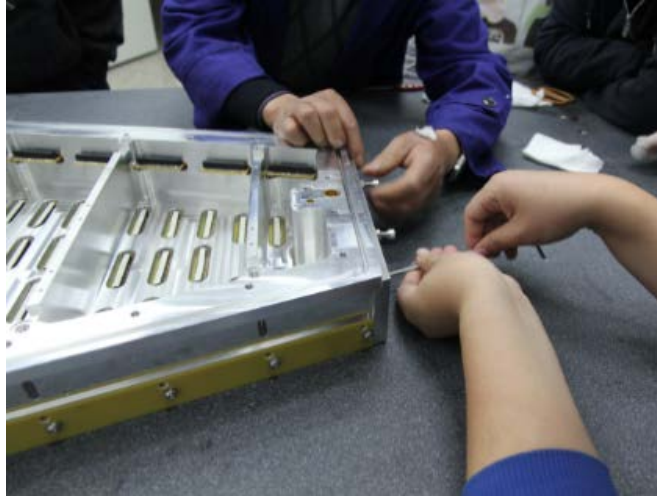
Figure 77: Attaching shield & gated wire mounts to strongback
