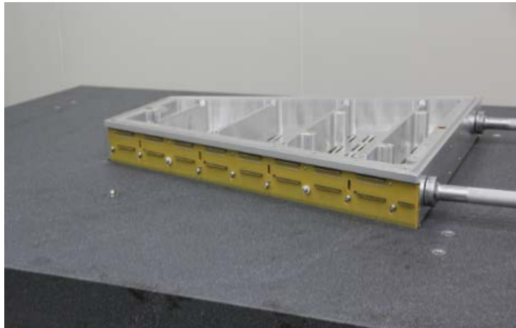
Figure 76: The anode wire mounts were glued to the strongback with epoxy..
