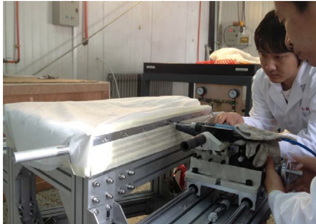
Figure 80: Drilling & pinning the side wire mounts
