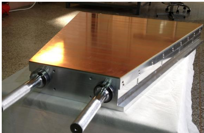
Figure 67: The strongback with the pad plane glued.
