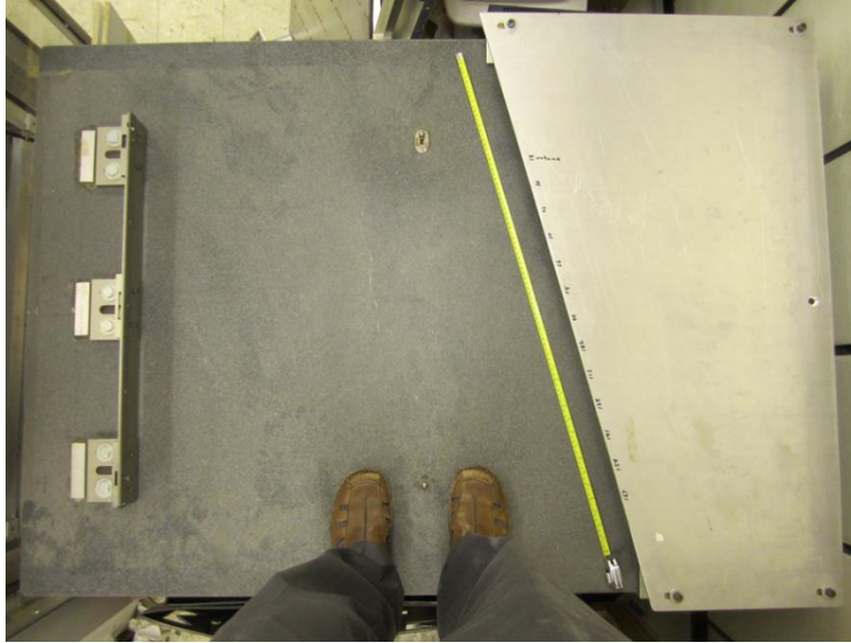
Figure 56: Top view of a granite table with one of the wire alignment combs exposed. The second comb lies under the aluminum shield on the right. Scale: the yellow portion of the tape is 1 meter long.
