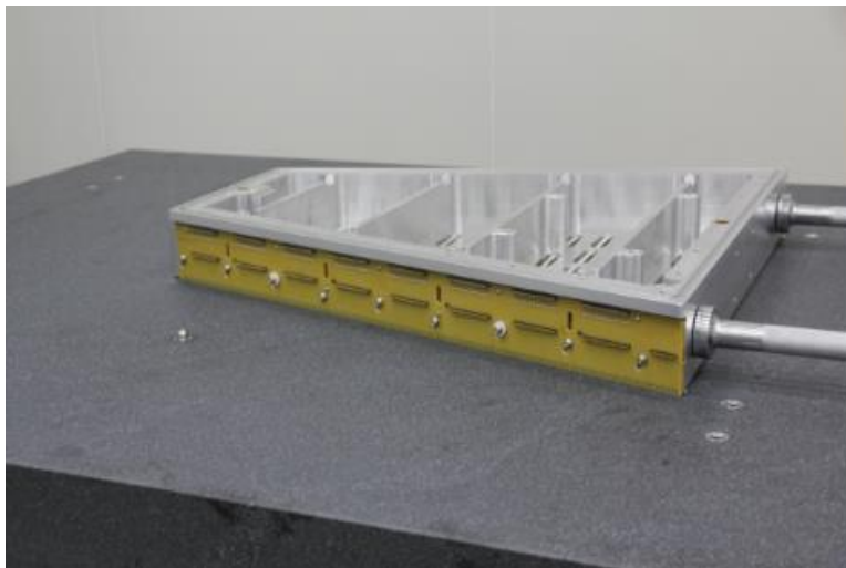
Figure 69: The anode wire mounts were glued to the strongback with epoxy.
