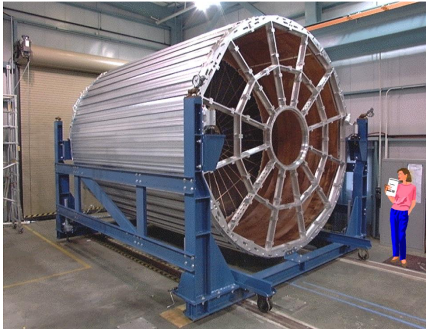
Figure 35: The STAR TPC during construction at LBL. The tracking volume of the TPC is 4 meters in diameter and 4.2 meters long. The photo shows how each end of the TPC is divided into 12 super-sectors and each super-sector is divided into an inner and an outer readout sector.
