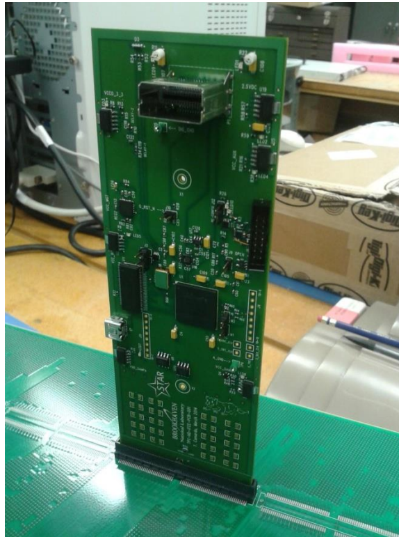
Figure 77: Pre-prototye iFEE (ppFEE) electronic card shown plugged into the padplane
