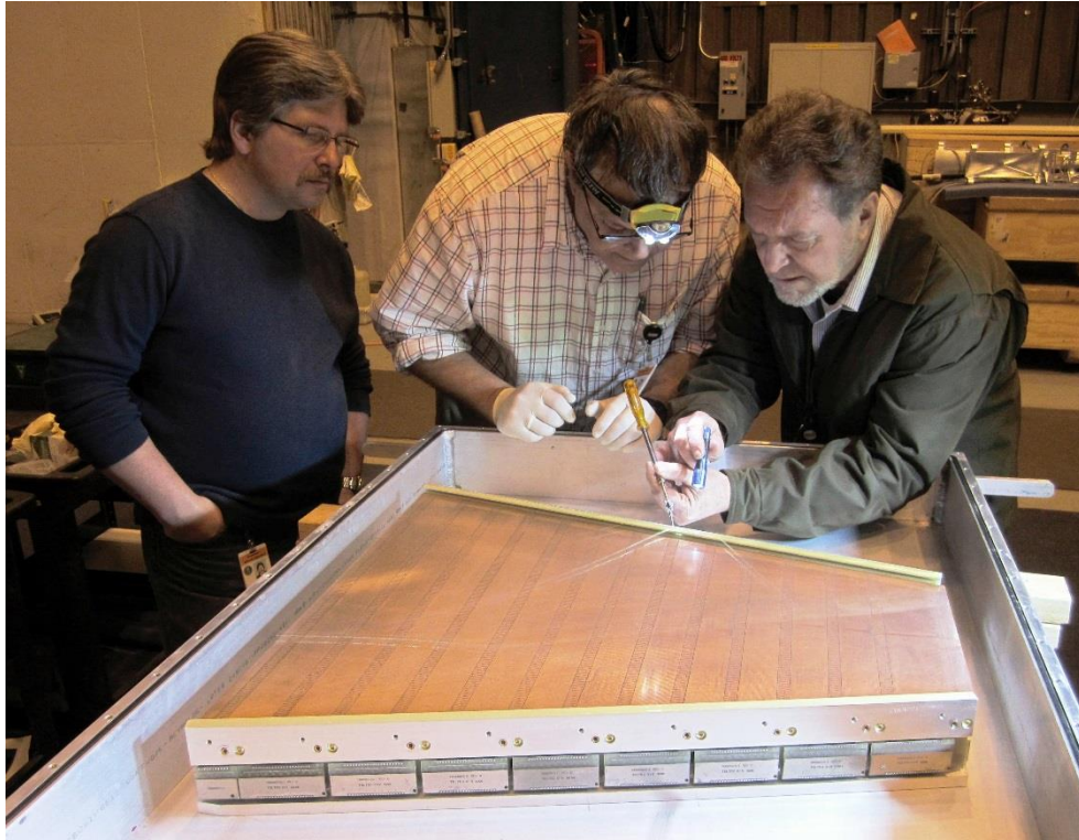
Figure 51: Experts examining a spare inner sector for the TPC. Note the old style padplane with electronics cards (ABDB boards) mounted along the edge of the sector. Normally the spare sectors (STAR has two spare sectors) are sealed in a storage box and kept under dry nitrogen.
