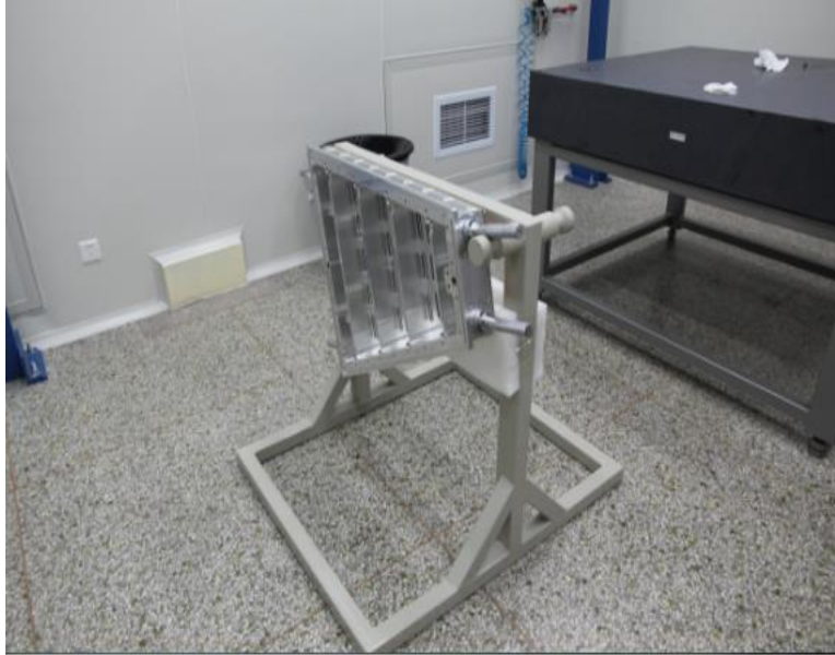
Figure 68: Gluing stand for anode wire mount and granite table.
