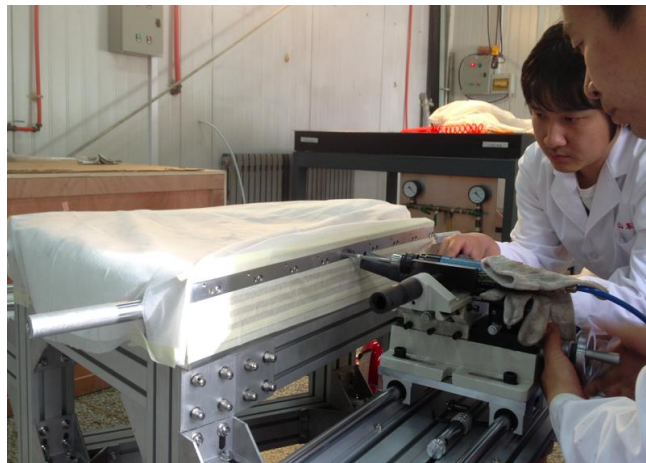
Figure 73: Drilling & pinning on side wire mounts
