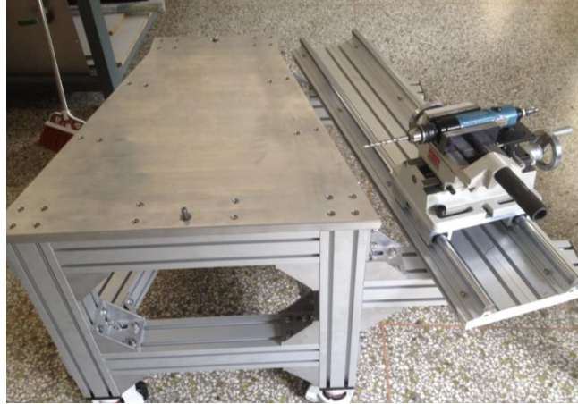
Figure 72: The drill/pinning fixture designed at SDU
