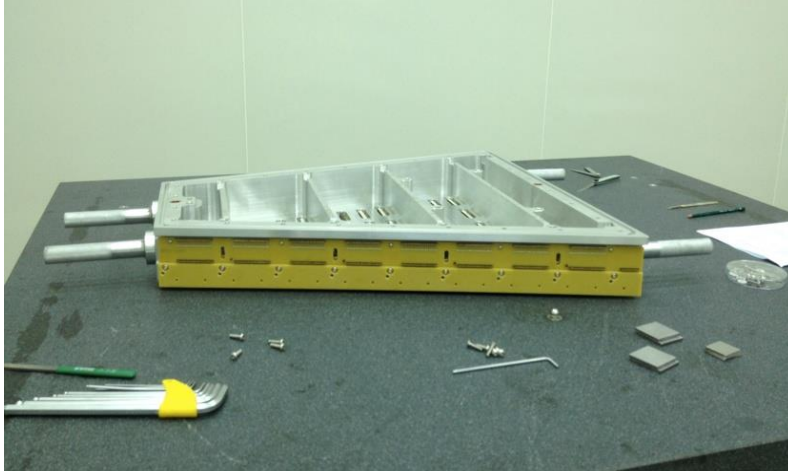
Figure 70: Attaching shield & gated wire mounts to strongback
