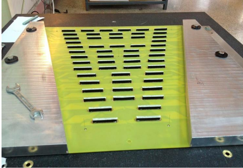
Figure 66: Padplane on granite table held flat by the suction of a vacuum system.
