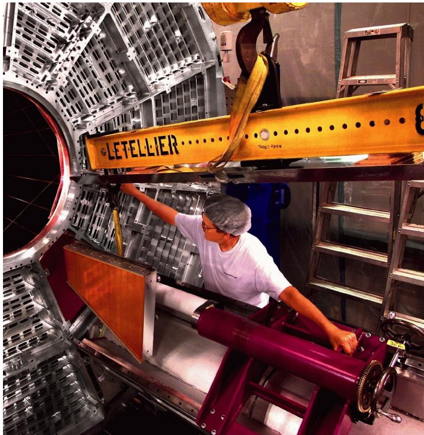
Figure 79: The original sector insertion tool. The sector must fit through the hole in the end-wheel, rotate, and finally pull back into place over a pair of alignment pins (tooling balls) that are located inside the TPC.
