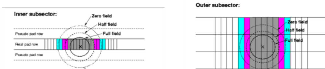
Figure 40: Simulations of the effective pad response function for pads on the inner and outer TPC padplanes. The inner pads were assumed to be 3.35 mm wide and the outer pads 6.7 mm wide. The circles show the 3-sigma limit for the pad response function convoluted with the diffusion limit for particles that drift the full distance from the CM to the padplane. P10 gas is assumed. The different circles show the different response that is recorded when the B field is set to 0.0, 0.25 T, or 0.5 T. [4]
