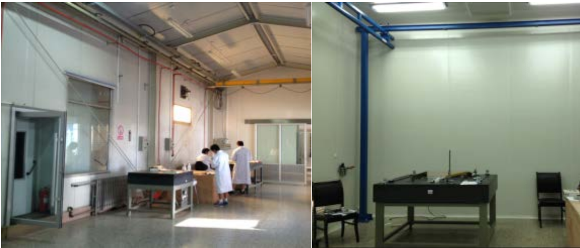
Figure 60: Experimental hall with two granite tables (left) and clean room with crane and granite table (right) for MWPC production at SDU.
