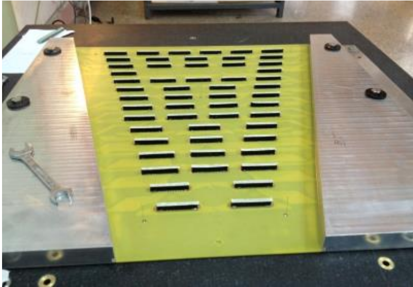
Figure 73: Padplane on granite table held flat by the suction of a vacuum system.
