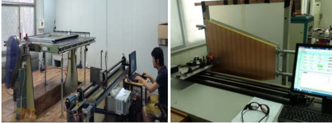
Figure 61: The wire winding machine at SDU (left) and the optical system for making wire tension measurements (right).
