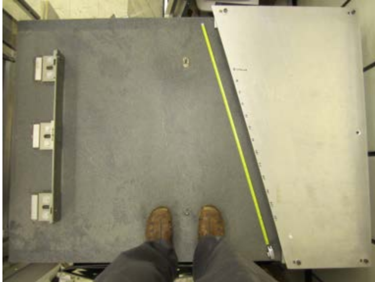
Figure 57: Top view of a granite table with one of the wire alignment combs exposed. The second comb lies under the aluminum shield on the right. Scale: the yellow portion of the tape is 1 meter long.
