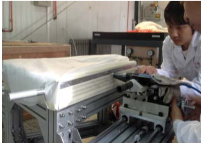
Figure 80: Drilling & pinning the side wire mounts
