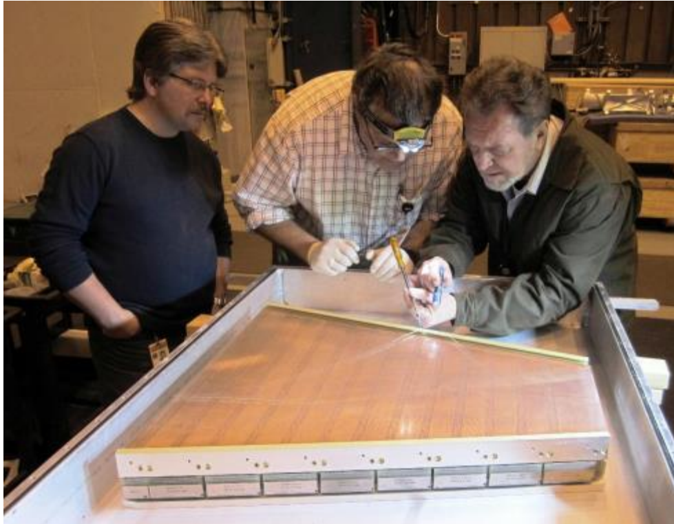
Figure 52: Experts examining a spare inner sector for the TPC. Note the old style padplane with electronics cards (ABDB boards) mounted along the edge of the sector. Normally the spare sectors (STAR has two spare sectors) are sealed in a storage box and kept under dry nitrogen.
