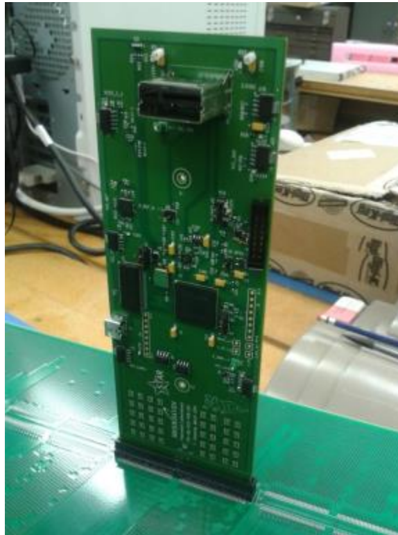
Figure 89: Pre-prototye iFEE (ppFEE) electronic card shown plugged into the padplane
