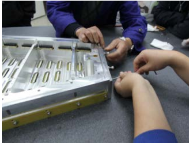
Figure 77: Attaching shield & gated wire mounts to strongback
