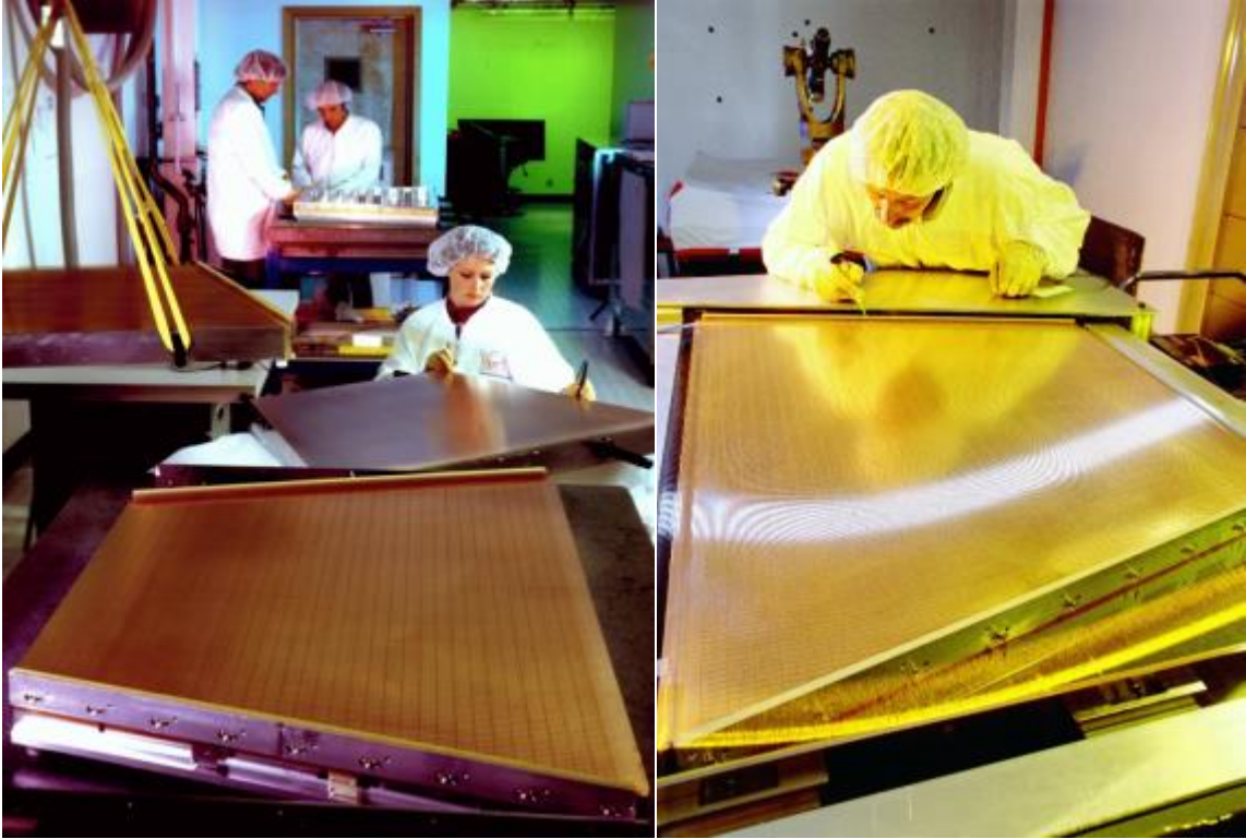
Figure 59: Outer sector MWPCs under construction in Berkeley (circa 1995).
