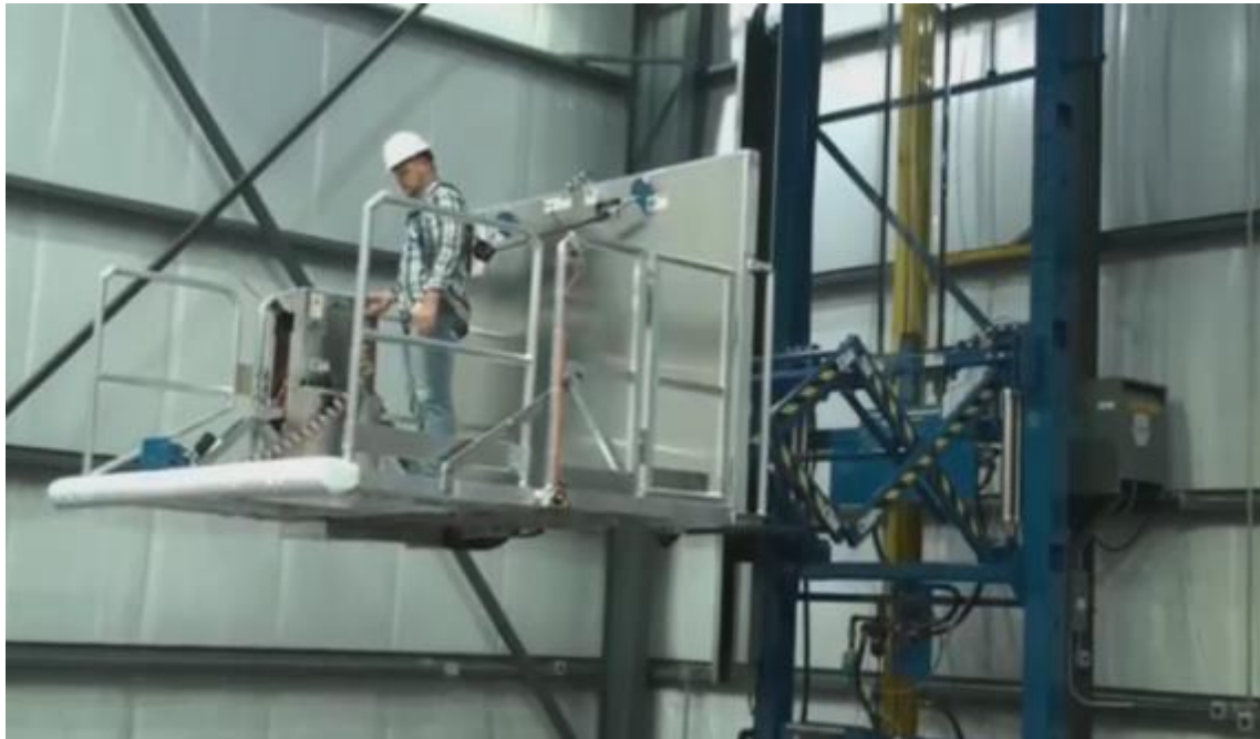
Figure 93: Photograph of an existing platform from Bastian Solutions. The lift in our particular application will not need the scissor extension in the horizontal direction.
