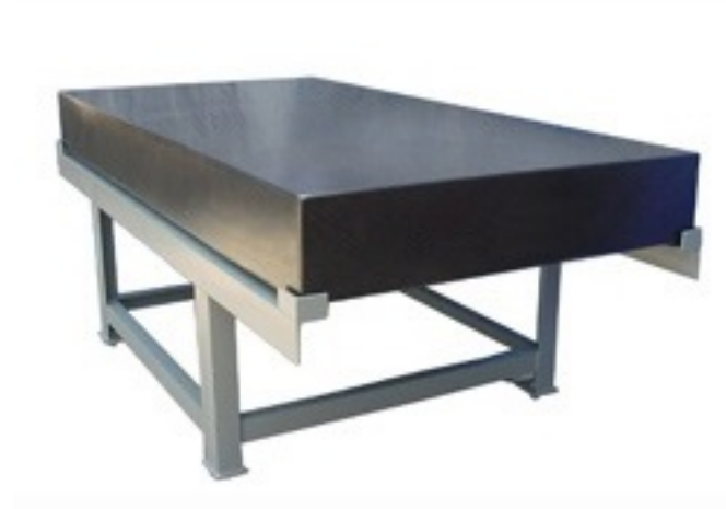
Figure 56: A typical Grade A inspection plate; otherwise known as a granite table. Typical dimensions are 6 feet by 4 feet by 8 inches, although the tables are available in many different sizes.
