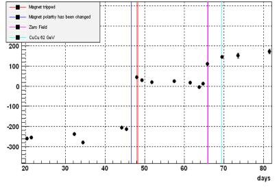
Lorentz effect: trajectory of electrons/holes are modified due to the combination of the STAR magnet B-field and the SSD wafer E-field
