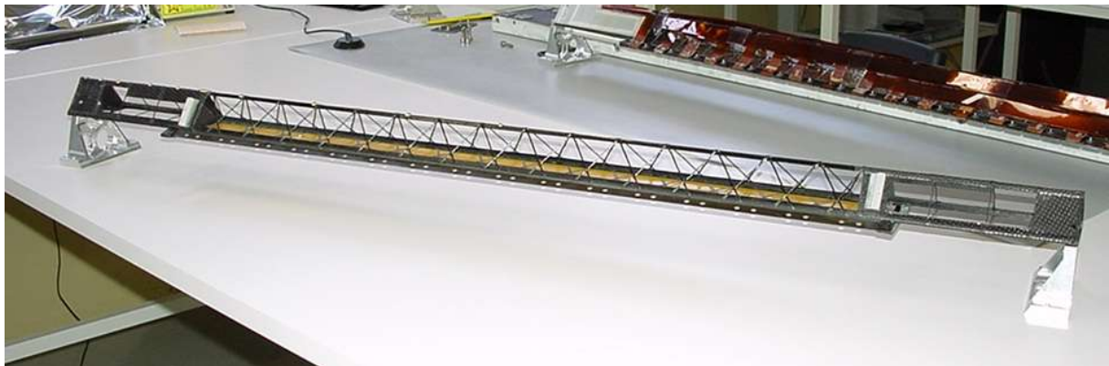
Figure 3 : a carbon fiber mechanical structure of a ladder
