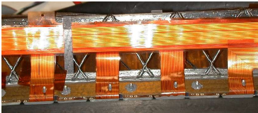
Figure 9 : Detailed top view of the ladder showing the aluminum buses connected to the hybrids and running along the ladder
