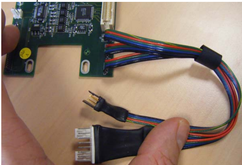
Figure 50: Power supply and sense pigtails (AWG24) and connectors for ADC card
