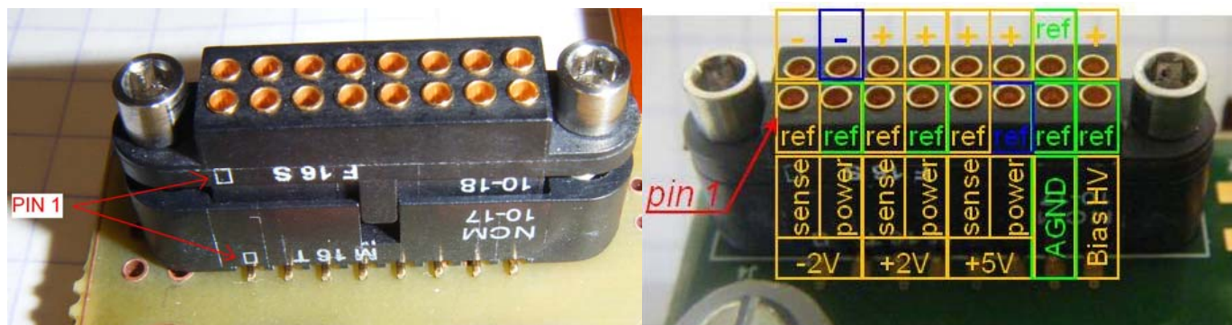
Figure 26: Nicomatic power connector cabling
