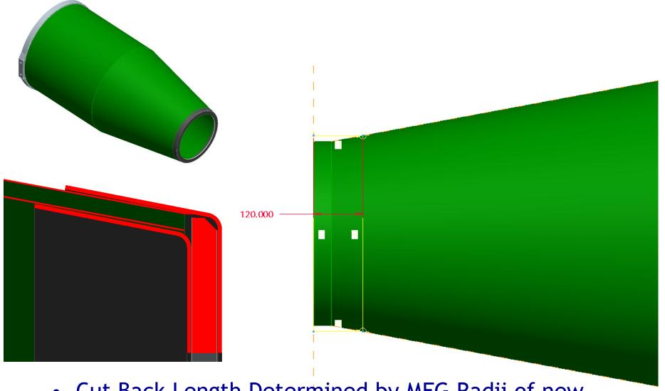
Cut Back Length Determined by MFG Radii of new Flanges—also allowance for Bolt Flange Radii
