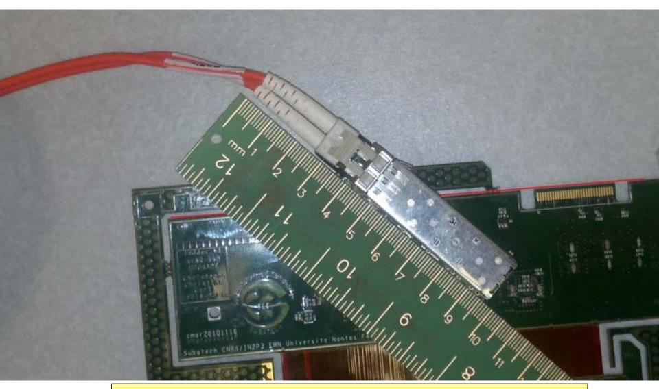
We need 5 cm beyond the top of the opto-coupler for fiber strain relief. Note: The red line is the top of the ladder card.
