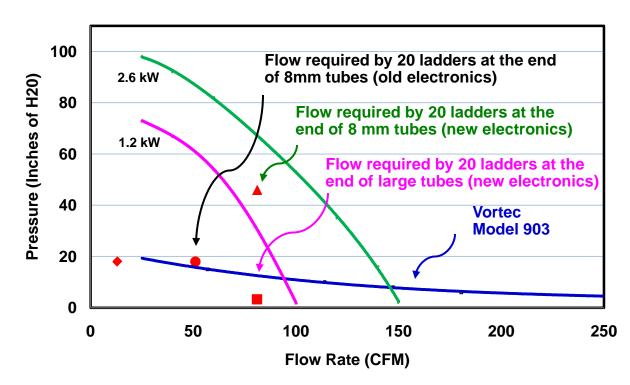
'Large tubes' means 4 long tubes with 2.5 cm (ID) each, then distributed locally to 20 ladders without additional pressure drop
