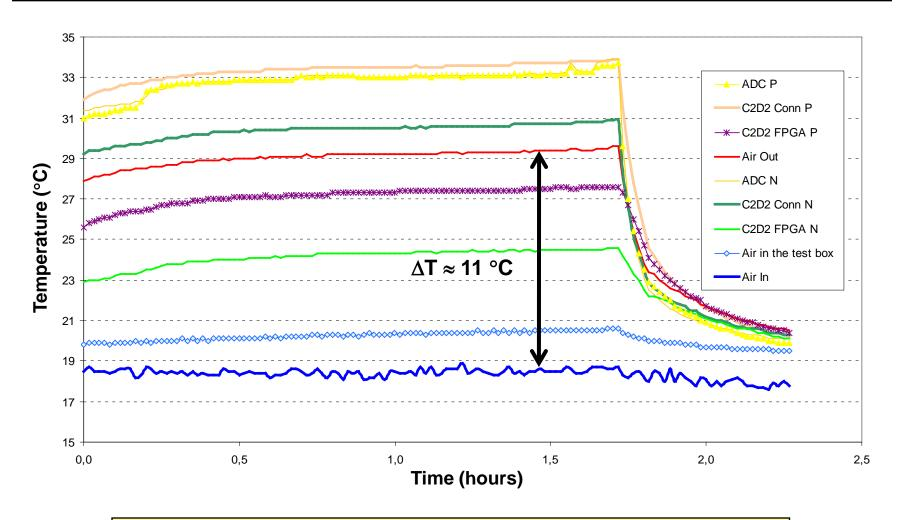
Measurements confirm that the majority of heat from the ladder is transferred to the cooling air stream. The system is efficient.
