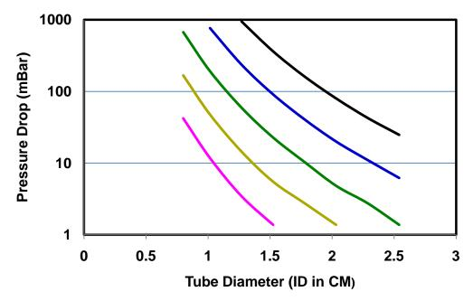
Pressure Drop as a function of diameter for constant flow rates of 1, 2, 4, 8 and 16 liters / second through a 4.5 meter long tube.
