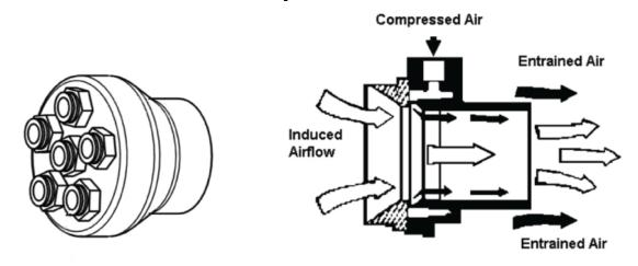
The left panel (above) shows the vacuum distribution manifold that transfers air from the small diameter tubes to the Transvector. The right panel shows the Transvector airflow amplifier and its principles of operation.
