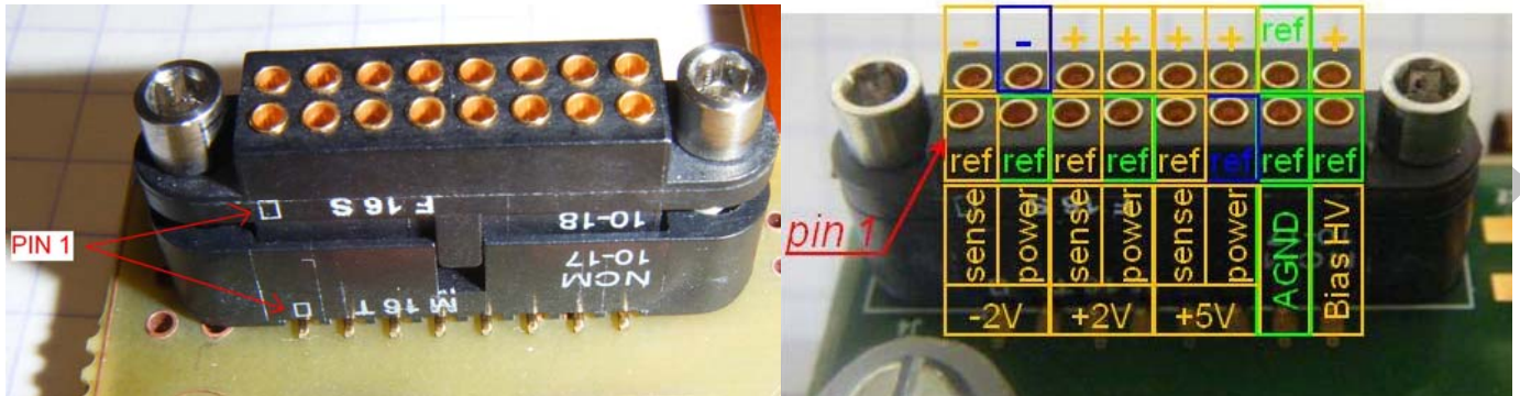
Figure 24: Nicomatic power connector cabling
