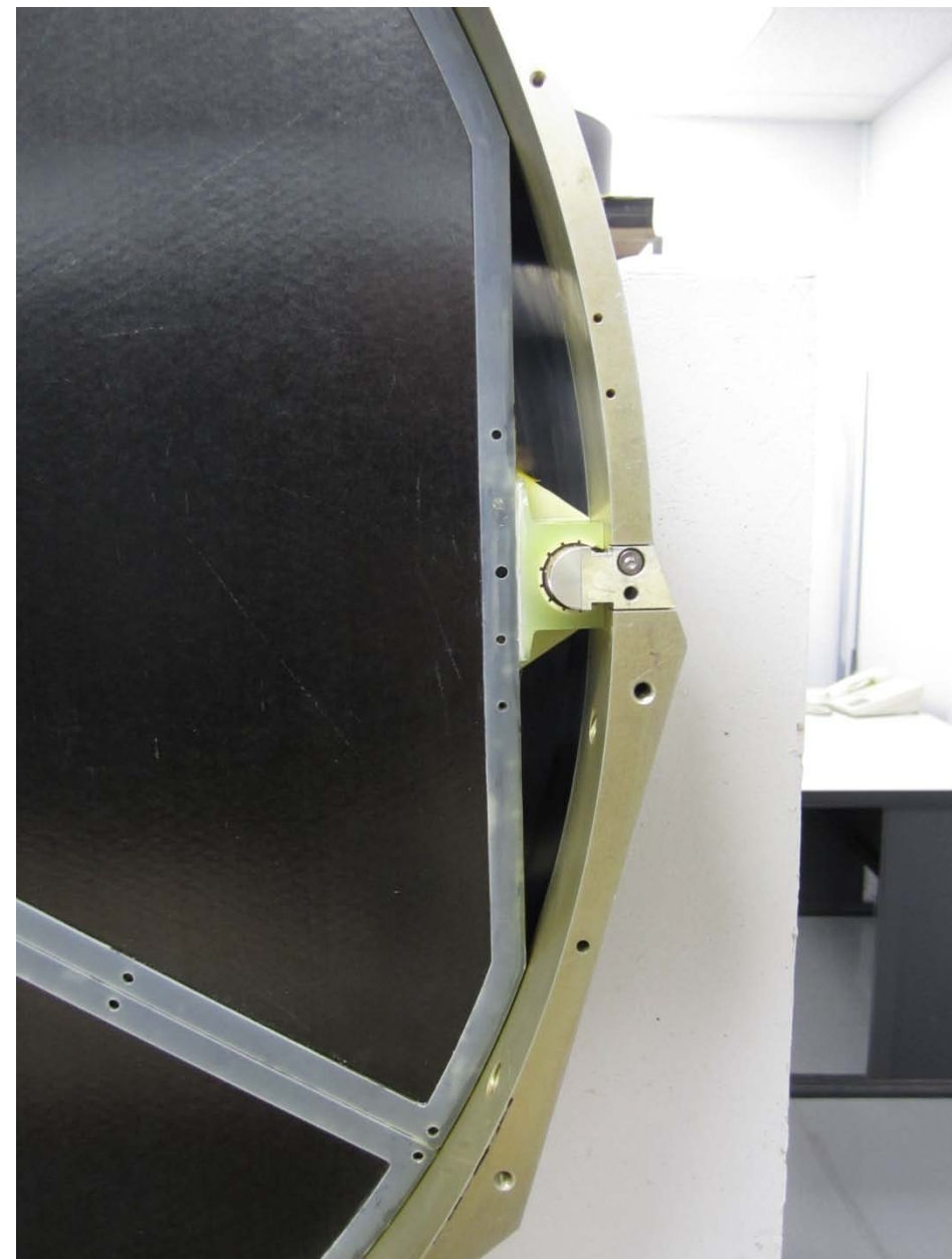
Space around the slider and rail is to be used for the SSD cables. Detail about rail as it goes into the cone. Rail is 2 cm in diameter.
