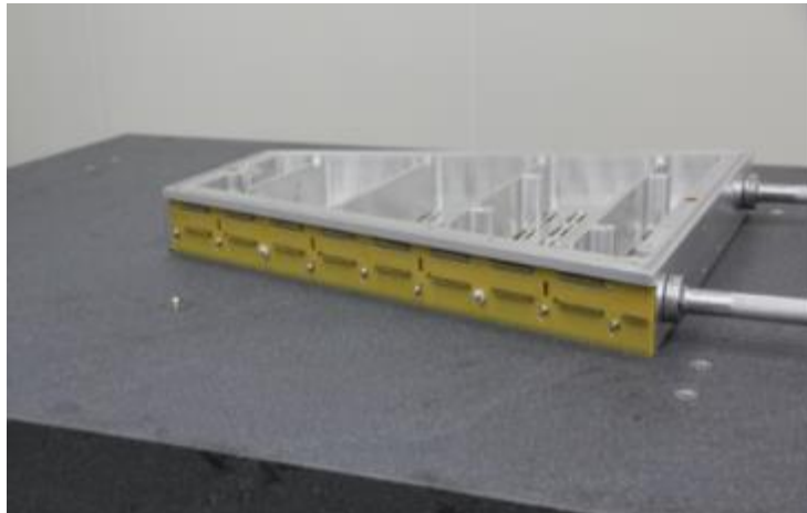
Figure 80: The anode wire mounts were glued to the strongback with epoxy..
