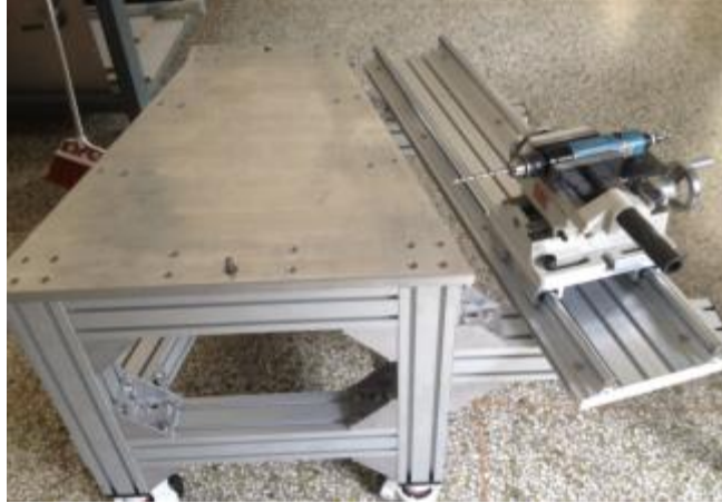
Figure 83: The drill/pinning fixture designed at SDU
