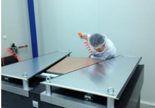
Figure 87: Epoxying the anode wires on the wire mounts with protecting covers in place.
