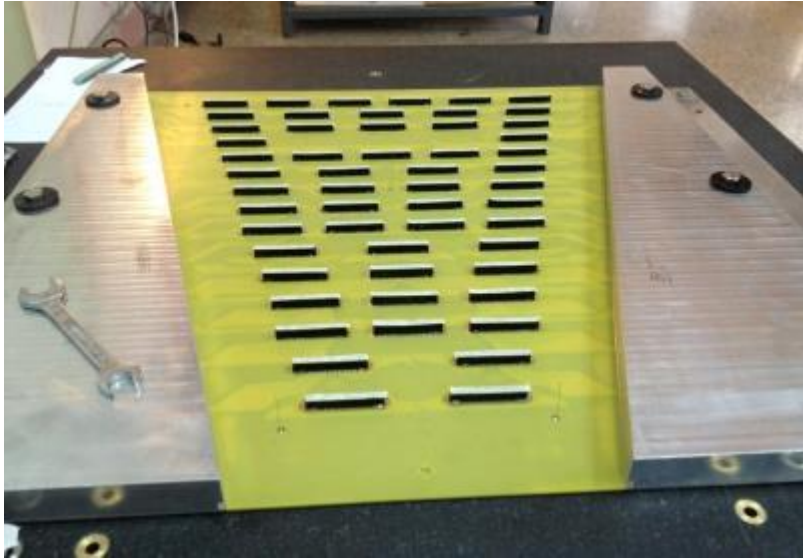
Figure 77: Padplane on granite table held flat by the suction of a vacuum system.
