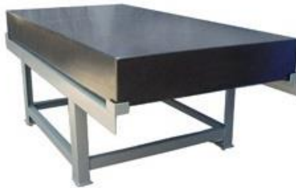
Figure 60: A typical Grade A inspection plate (otherwise known as a granite table). Typical dimensions are 6 feet by 4 feet by 8 inches, although the tables are available in many different sizes.
