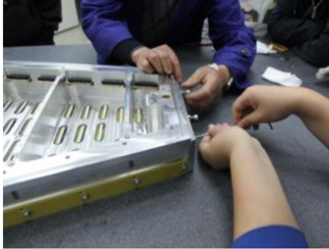
Figure 81: Attaching shield & gated wire mounts to strongback
