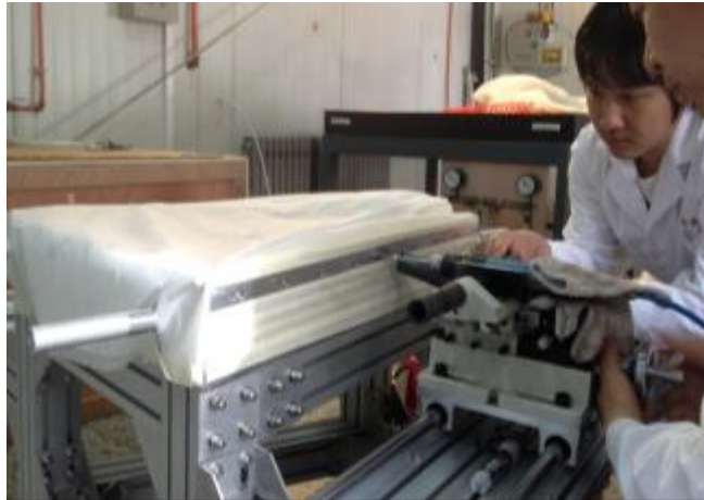
Figure 84: Drilling & pinning the side wire mounts
