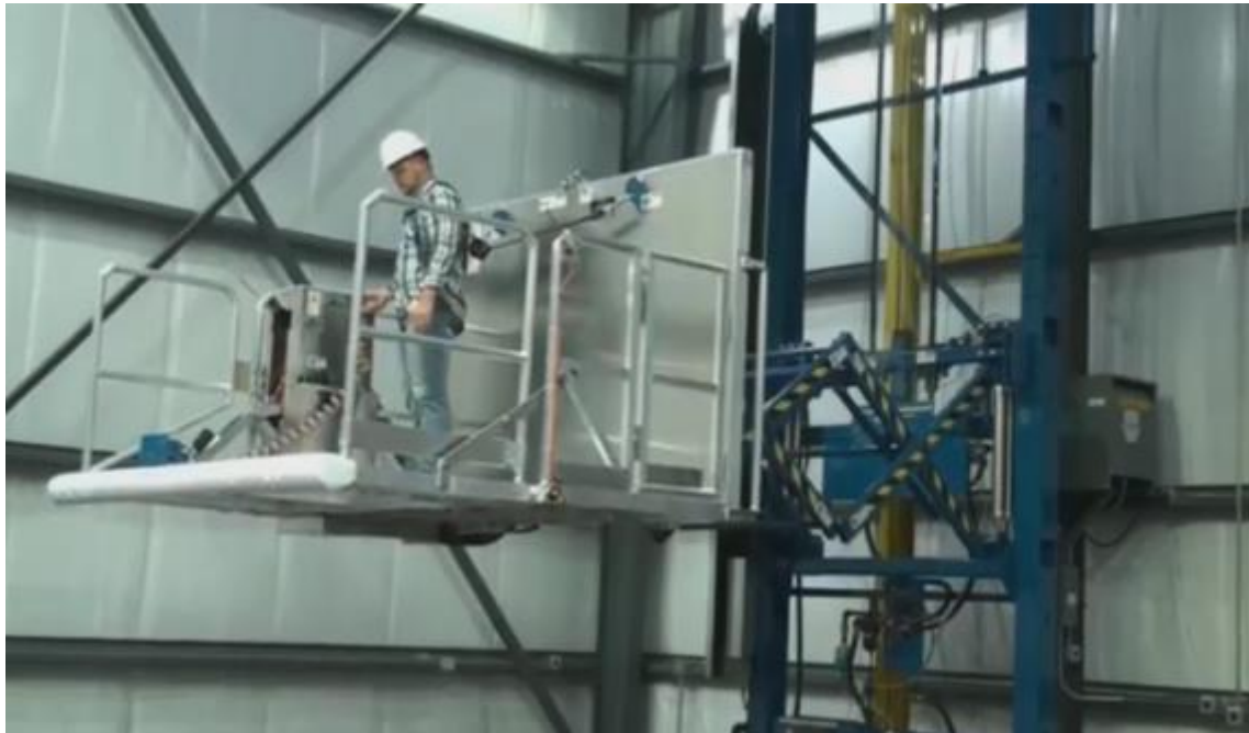
Figure 95: Photograph of an existing platform from Bastian Solutions. The lift in our particular application will not need the scissor extension in the horizontal direction.
