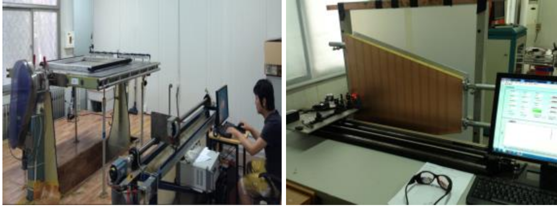
Figure 65: The wire winding machine at SDU (left) and the optical system for making wire tension measurements (right).
