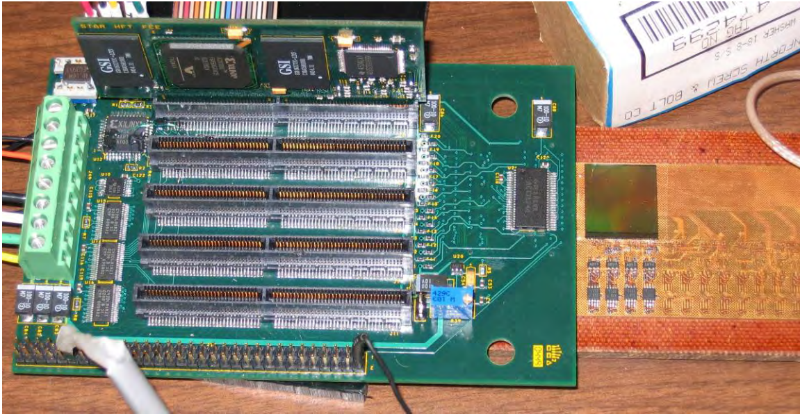
Figure 48: Early Prototype motherboard and daughter card used for reading out MIMOSA5 detectors.
