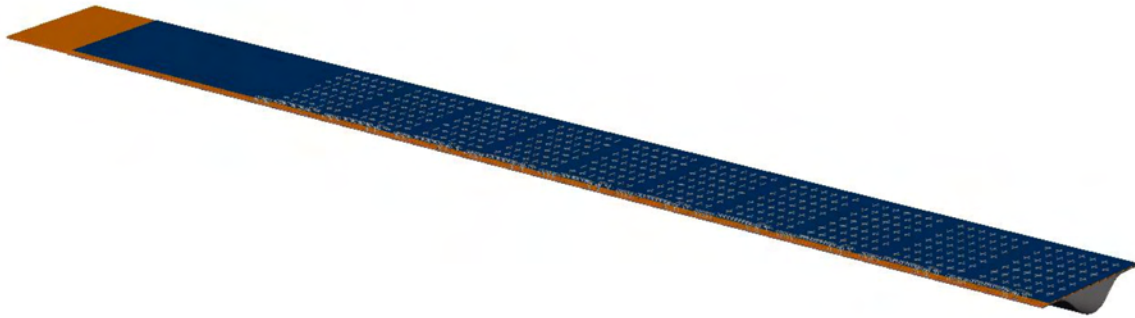
Figure 54: Ladder assembly. The current ladder is composed of a row of 10 thinned APS detectors on top of a matching row of thinned readout chips and a three-layer aluminum Kapton cable. The silicon cable structure is bonded to a carbon composite “v”, closing the beam to make a rigid structure.
