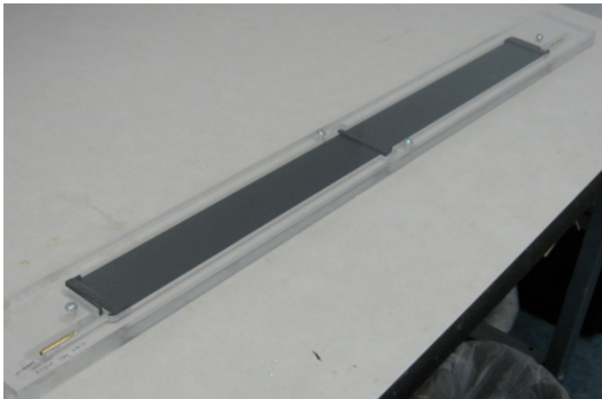
Figure 62: Long IST prototype ladder made out of carbon fiber honeycomb and carbon fiber skins. This prototype has one cooling channel.
