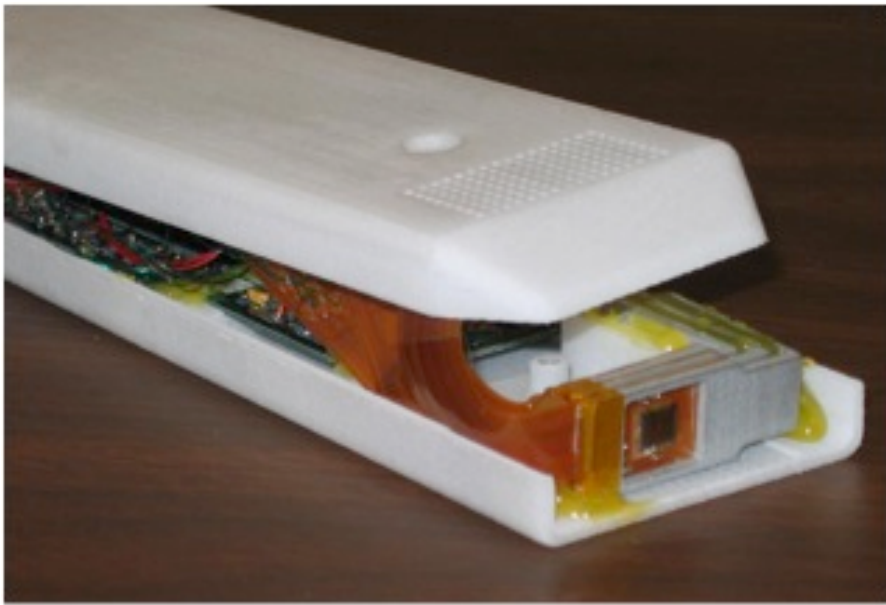
Figure 53: Three Mimostar-2 sensors in the telescope configuration used in the beam test at STAR.
