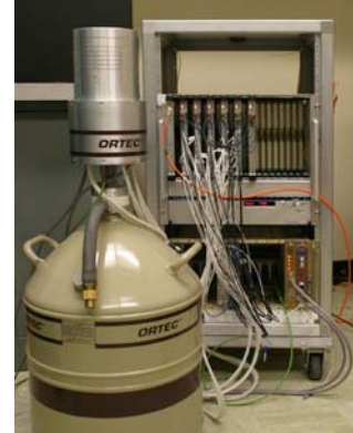
Figure 2: The detector in its cryostat and with its DAQ electronics
