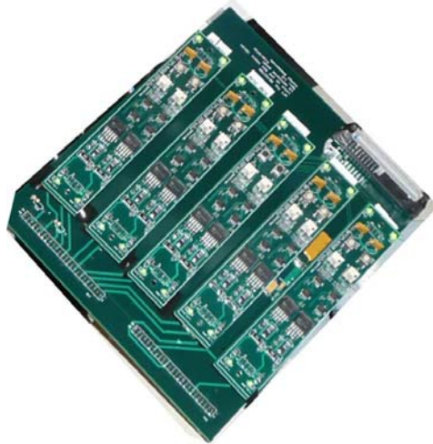
Figure 2 A set of 10 LU-monitoring power supply modules that were built for the PXL detector development is shown attached to a dedicated support PCB; there are five modules on each side of the PCB. Each module provides two latchup-monitored, independent power supply channels.
