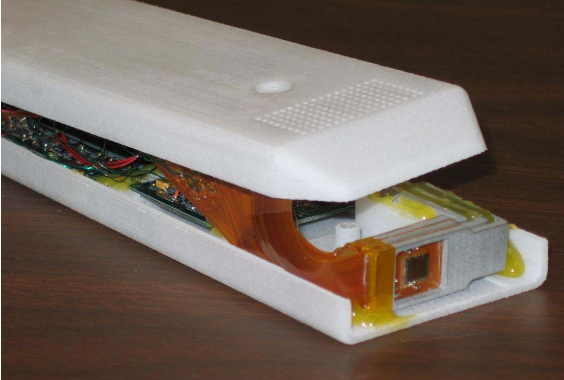
Figure 2: Picture of three sensor Mimostar2 telescope mounted in the plastic housing head.
