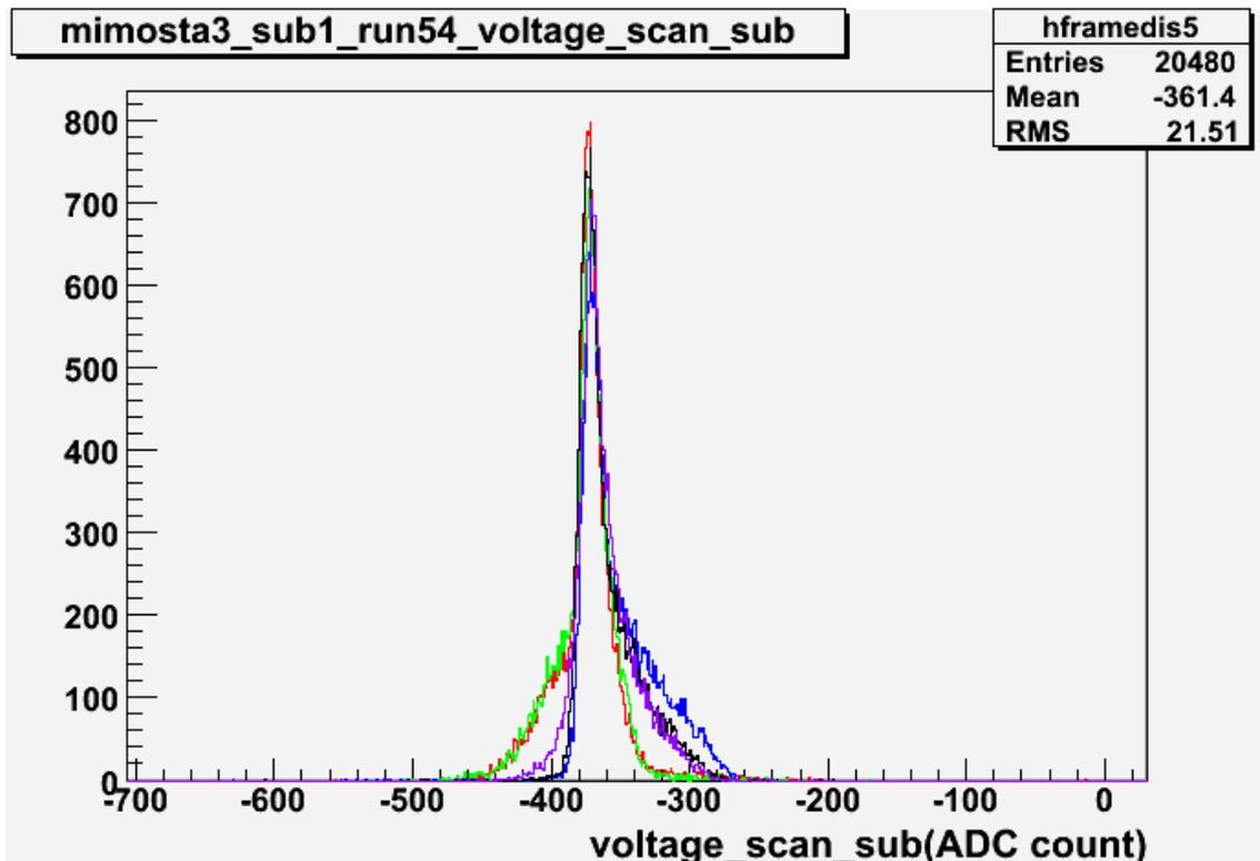
Figure 8 Histograms of smaller sub-arrays based on each of the 5 gain=3/5 amplifiers in sensor sub-array 0 at the gain=3 setting
