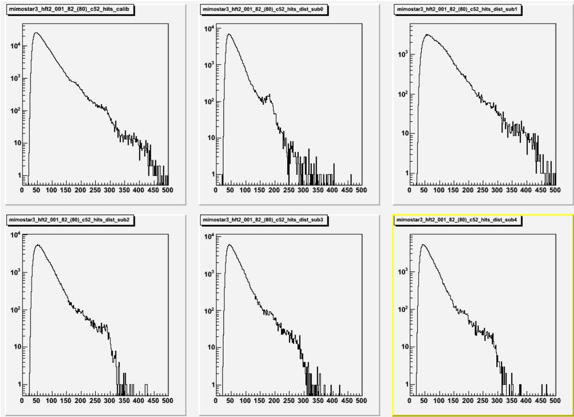
**Figure 3**  $^{55}\text{Fe}$  calibration peak distributions for 5 sub-arrays analyzed together and separately for sensor A4 and the internal gain=5.
