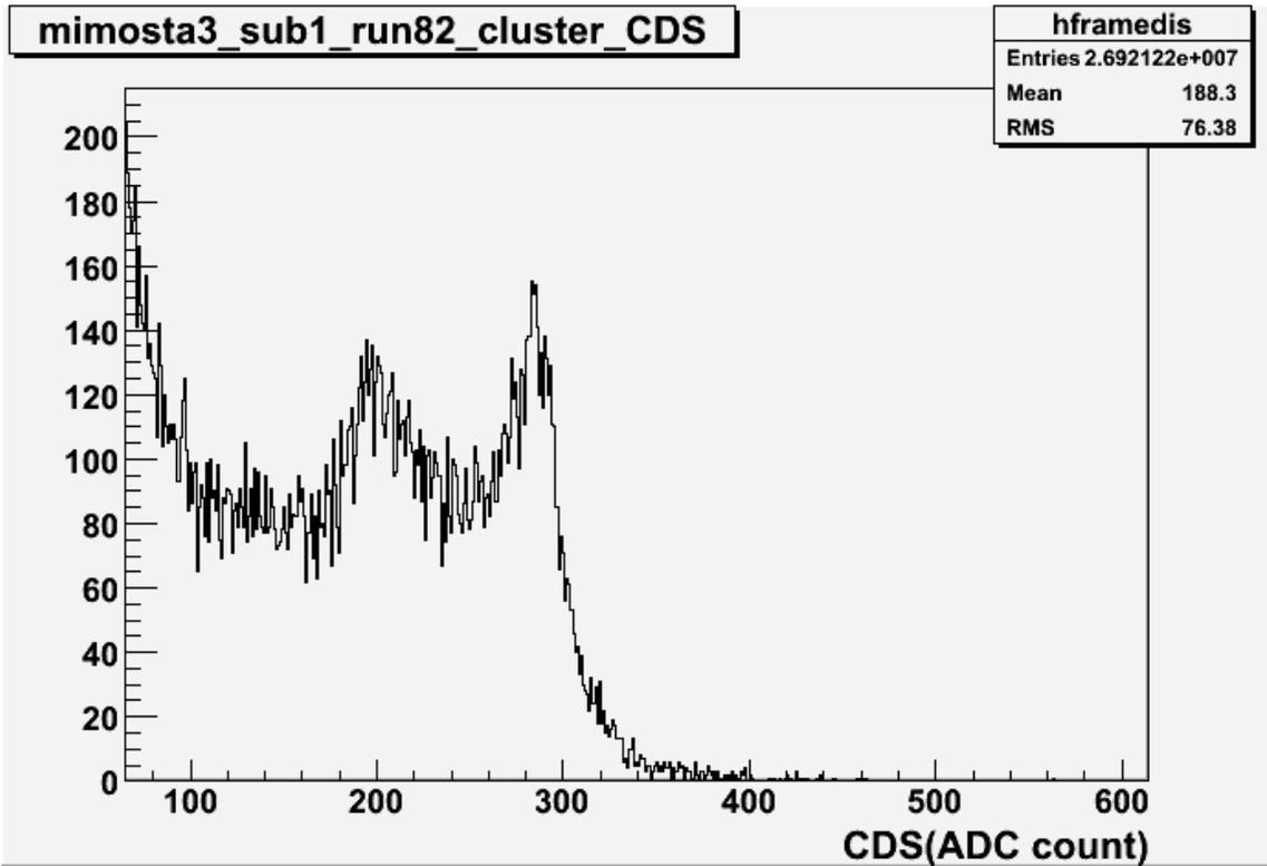
Figure 5 Sensor A2 raw CDS spectrum on gain=5 setting with XS cuts analysis (zoomed)
