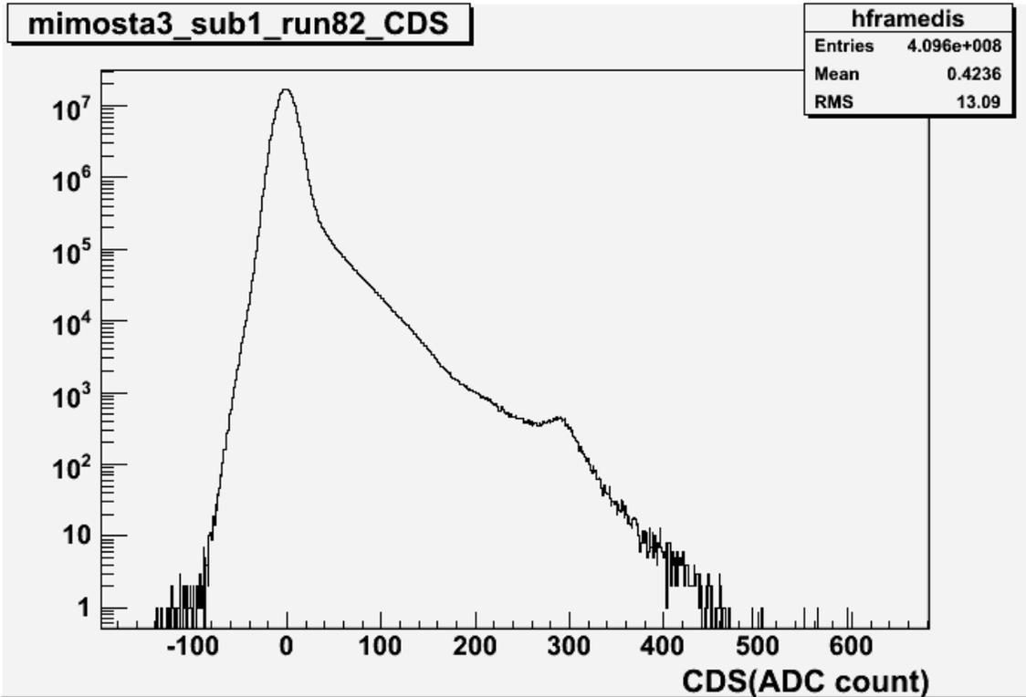
Figure 4 Sensor A2 raw CDS spectrum on gain=5 setting
