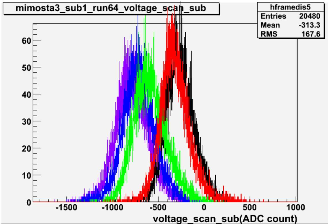
Figure 7 Histograms of smaller sub-arrays based on each of the 5 gain=3/5 amplifiers in sensor sub-array 0 at the gain=5 setting
