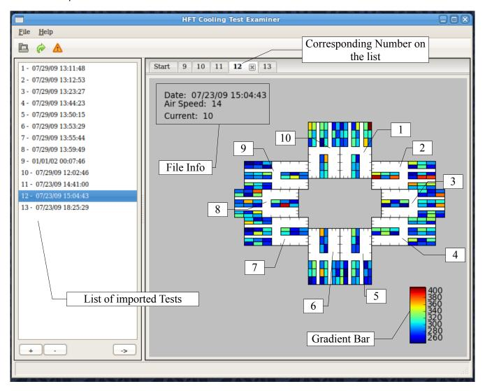
Each number in the picture above identifies the corresponding module that was tested. This graph maps to the physical device if you look at it from the wired end. Each ladder is represented by the set of 6 rectangles, and each rectangle is corresponding thermistor. The ladder closest towards the middle in the graph represents the inner ring of thermistors, and the outer ring is the rest of them in order.
