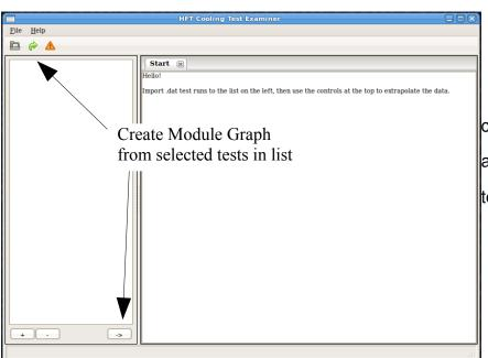
Click these buttons to create a new graph showing all the modules in the selected test runs.
