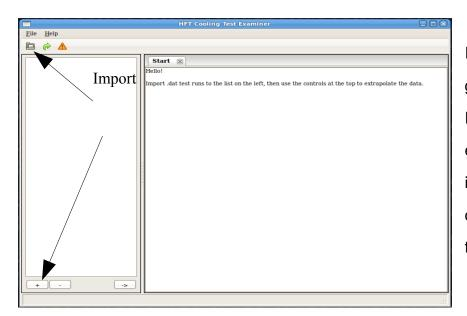
Import .dat files generated by the Tester Program by clicking either of the buttons indicated in the picture on the left or through the file menu, "import".
